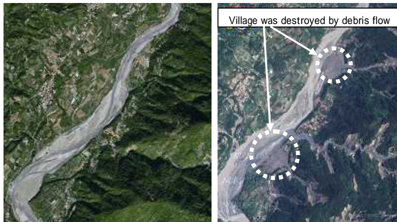
Figure-7: Sinkai Village and Sinfa Village with their communities engulfed by a debris flow (left: before the disaster)
